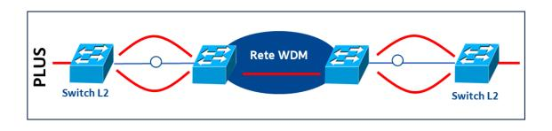
• **Top** Single connection where E2E protection is realised, with two separate ways along the entire path of the connection:
