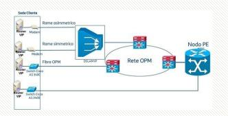
A router (VIP router provided on a rental and maintenance basis) is installed for each VIP network connection to manage VIP IP traffic. IP service traffic is processed using Classes of Service (CoS), which allow traffic to be prioritised according to the three classes of descending importance described below:
